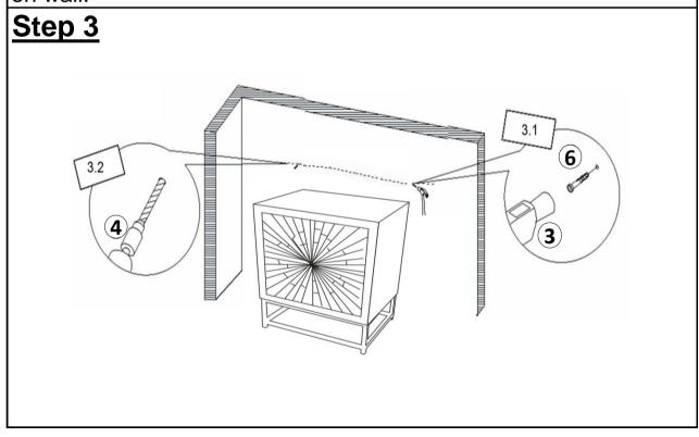
3.1) Drill two holes on wall at 5 cm below from the height of bedside as Metal Brackets (9) on Bedside with Power Drill (4).
