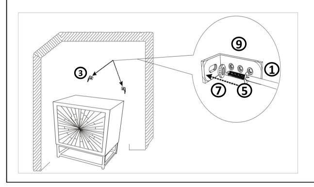
Attach Brackets (9) to Wall Plugs (6) using Wall Plug Screws (5) and washer (7) with Screwdriver (1).
