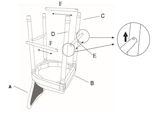
Insert the Side Stretchers(F) and the Front Stretcher(E) into the mounting positions between the legs in sequence.
