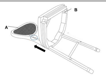
Attach the two slots on the Chair Seat(B) to the lower legs on the Chair Back(A), then push the Chair Seat(B) upward to align it with the mounting positions on legs.
