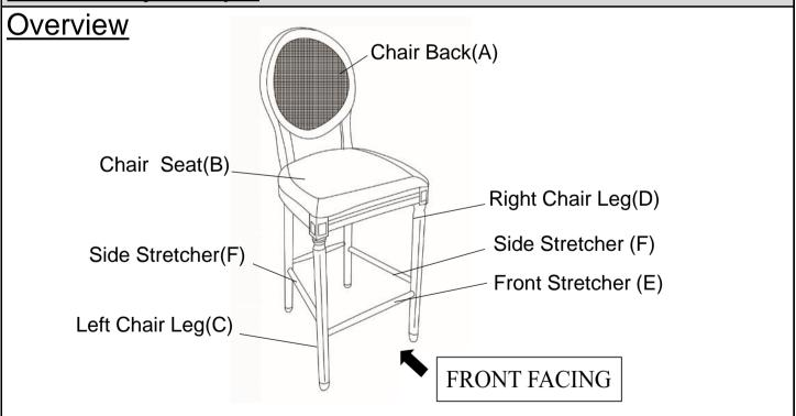
This Bar Stool has multiple parts and may require up to 30 minutes to assemble. To give you an overview of the Bar Stool parts, the above picture is provided to help you put the various parts into perspective. Please read through the instructions below to familiarise yourself with the parts and steps before assembly.
