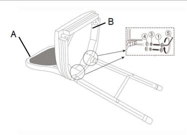
With assistance from a second adult, attach the Chair Seat(B) to the Chair Back(A) using Bolts(①), Spring Washers(③) and Washers(④) with the Allen Key(⑤).
