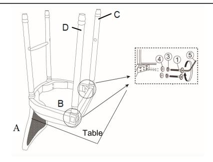
Place the assembled Chair Back(A) and the Chair Seat(B) downward on a clean, non-marring table. Attach the Left Chair Leg(C) to the Chair Seat(B) using Bolts(1), Spring Washers(3) and Washers(4) with the Allen Key(5).
