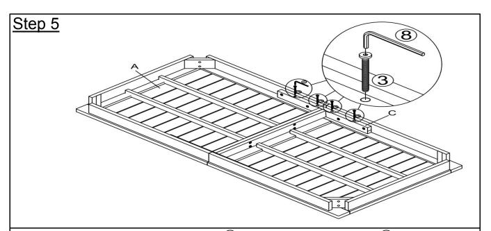
Loosely affix it vertically, using Bolts(3) with the Allen Wrench (8), as shown in the picture
