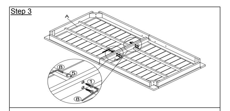
Affix the two parts of the Foldable Table Top (A) together using Bolts( $\widehat{\ }$ ), Nuts ( $\widehat{\ }$ ) with the Allen Wrench ( $\widehat{\ }$ 8) as show in the above picture. **Do not Fully tighten the Bolts.**
