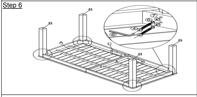
Attach the Leg (B) to the mounting position at the corrner of the Foldable Table Top (A), using the Bolts(4), Spring Washers (6), Flat Washers (7) with Allen Wrench (8).
