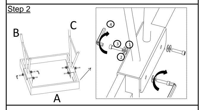
Place the Top (A) upside down onto a clean, soft surface to avoid any scratches or damages to the product. Align the holes of Top Panel (A) into All legs (B) as shown above. Then, affix the Top Panel (A) with legs (B) by using Washer (1), Lock Washer (2), Allen Screw (3) with help of Allen key (4).
