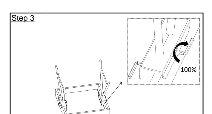
Tighten all the screws 100% with the help of Allen key (4).
