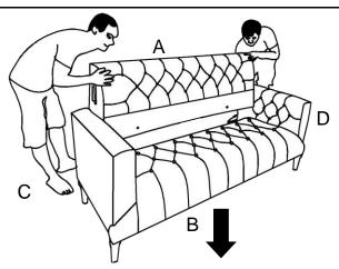
Make sure both sides of Backrest (A) at the same height and align the mounting brackets of it with those on the both arms synchronously, meanwhile use your knee to push the arms close to the Backrest(A) and push it downwards (until mounting brackets join together),make sure the top side at the same level as the Left Arm(C) and Right Arm(D)
