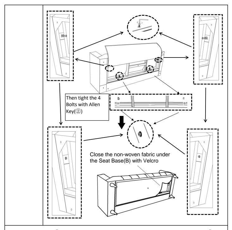
Using the Allen Key(2) secure Backrest(A) to the bottom of Seat Base(B) with Bolts(4), Spring Washers(3) and Washers(4).
