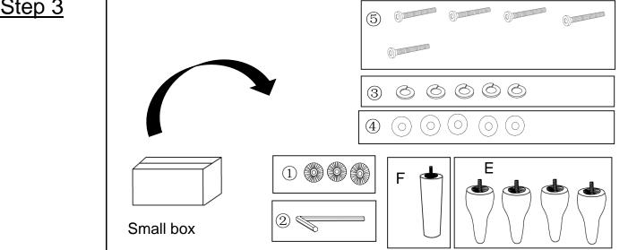
Open the Small Box to take out the Plastic Gasket(1), Allen Key(2), Spring Rings(3), Flat Gasket(4), Bolts(5), Legs with Plastic Gasket(E) and Middle Leg with 1 Plastic Gasket.
