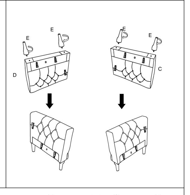
Carefully install the Wooden Legs(E) at the bottom of Left Arm(C) and Right Arm(D). Insert threaded stem into the mounting position at the corner of Left Arm(C) and Right Arm(D). Tighten by turning the Legs clockwise.
