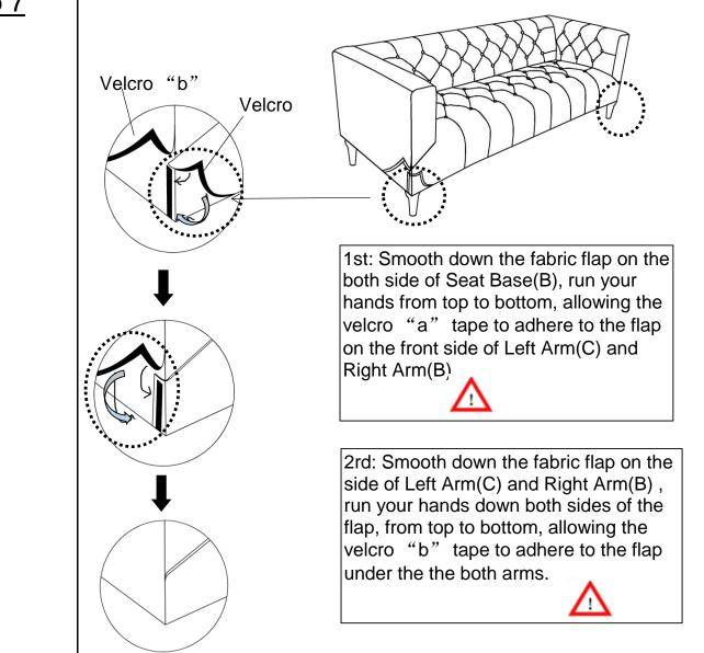
1st: Smooth down the fabric flap on the both side of Seat Base(B), run your hands from top to bottom, allowing the velcro "a" tape to adhere to the flap on the front side of Left Arm(C) and Right Arm(D).
