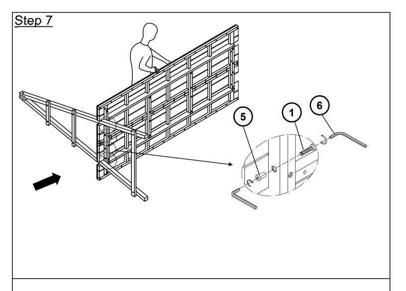
With the help from your adult partners, attach the Finished Leg Frame to the Table Tops using Bolts(1) and Sleeve Nuts(5) with Allen Keys(6) as pictured above.
