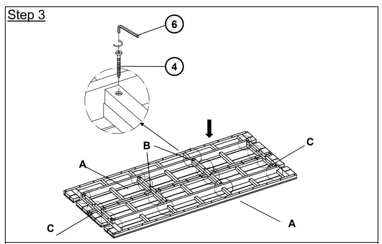
Attach Table Top Middle Support Bars(B) and Table Top Side Support Bars(C) to Table Tops(A) using Screws(4) with Allen Key(6) as pictured above.
