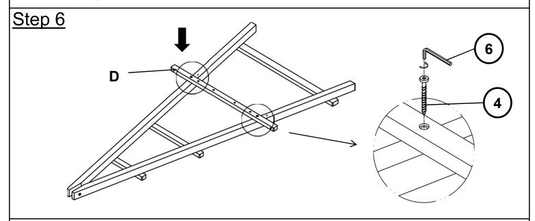
Attach Table and Leg Support Bars(D) to Legs using Screws(4) with Allen Key(6) as pictured above.
