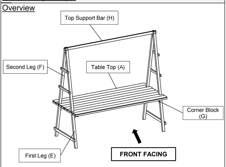
This Table has multiple parts and may require up to 30 minutes to assemble. To give you an overview of the Table parts, the above picture is to help you put the various parts into perspective. Please read through the instructions below to familiarise yourself with the parts and steps before assembly.
