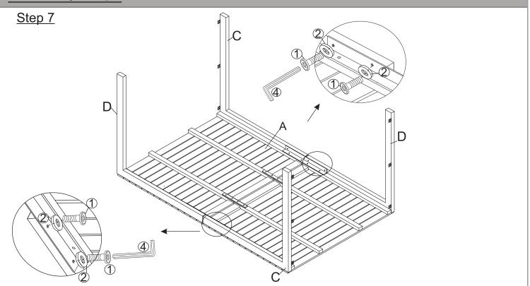
Repeat the same process in step 5 and step 6 with the other 2nd Leg (C) and 3rd Leg (D) **Do not fully tighten the Bolts.**
