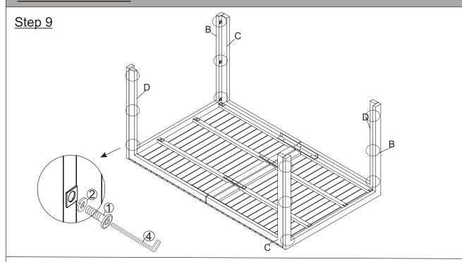
Attach the 1st Legs (B) to the 3rd Legs (D) and 2nd Legs (C) using Bolts (1) with Washers (2) and Allen Key (4), as show in picture above. Do not fully tighten the Bolts.
