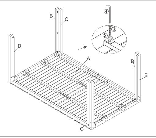
Attach the 1st Legs (B) to the short side of Table Top (A) using Screw (③) with Washers (②) and Allen Key (④), as show in picture above.
