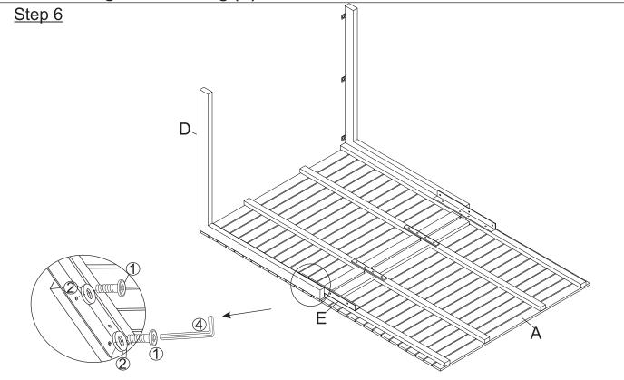
Place the 3rd Leg (D) to the long side of Table Top (A) and Support Bar (E), secure by using the Bolts (1), Washers (2) and Allen Key (4) as shown in the picture. Do not fully tighten the Bolts.
