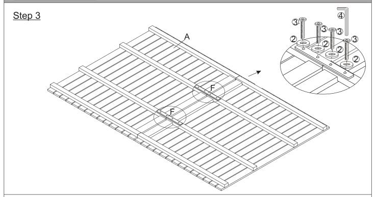
Place Middle Support Bar (F) to the housings of Table Top (A), secure by using the Screw (3), Washers(2) and Allen key (4), as shown in the picture. **Do not fully tighten the Screws.**
