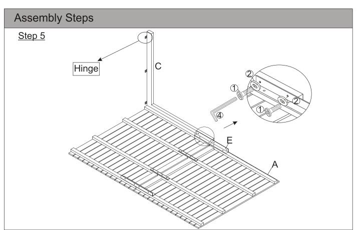
Place the 2nd Leg (C) to the long side of Table Top (A) and Support Bar (E), secure by using the Bolts (1), Washers (2) and Allen Key (4) as shown in the picture. **Do not fully tighten the Bolts.**
