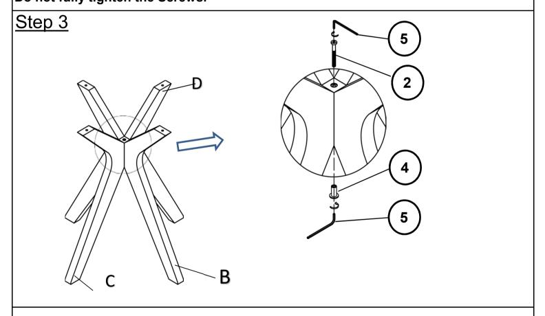
Then, attach First Leg(B) to Second Leg(C) and Third Leg(D) using Bolt((2)) and Sleeve((4)) with Allen Keys((5)).
