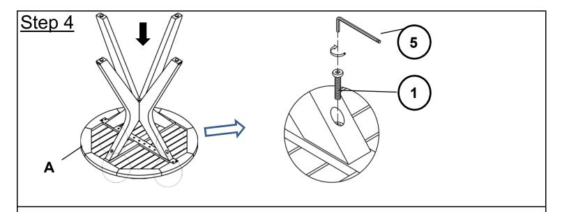
Attach Leg Frame to the Table Top(A) using Bolts( $\widehat{1}$ ) with Allen Key( $\widehat{5}$ ). **Do not fully tighten the Bolts.**
