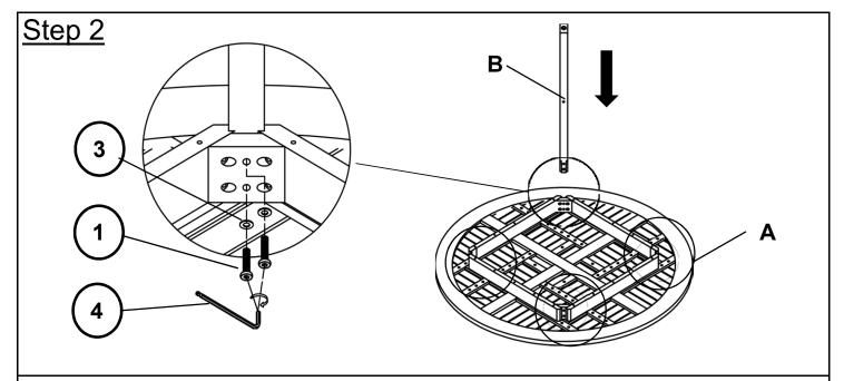
Attach Leg(B) to the Table Top(A) using Bolts( $\widehat{1}$ ), and Washers( $\widehat{3}$ ) with Allen Key( $\widehat{4}$ ). **Do not fully tighten the Bolts.**
