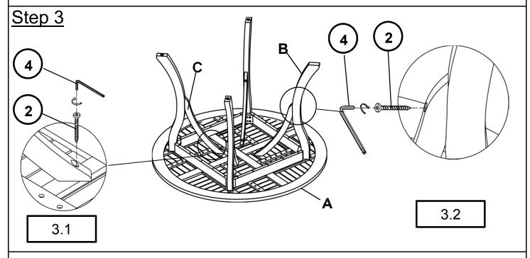
Place Leg Supports(C) between Table Top(A) and Leg(B), as shown above.
