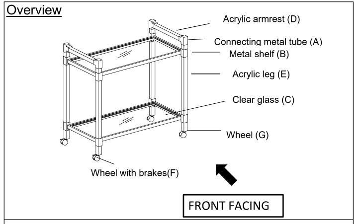
This Bar Cart has multiple parts and may require up to 30 minutes to assemble. To give you an overview of the Bar Cart, the above picture is to help you put the various parts into perspective. Please read through the instructions below to familiarise yourself with the parts and steps before assembly.
