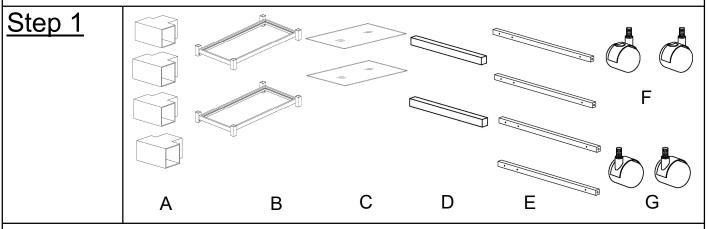
Place the Connecting metal tube(A), Metal shelf (B), Clear glass (C), Acrylic armrest (D), Acrylic leg (E), Wheel with brakes(F) and Wheel (G) on a clean, non-marring surface.
