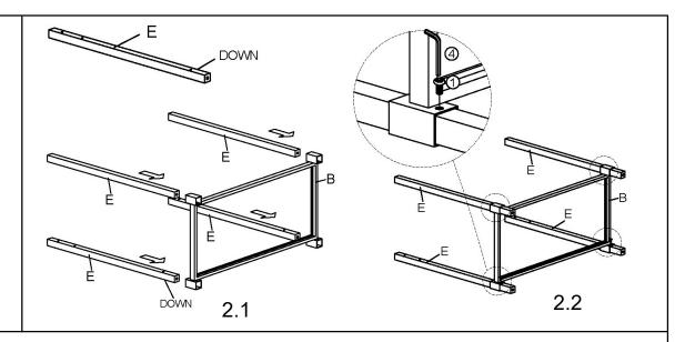
**2.1)** Insert the Acrylic legs (E) to Metal shelf (B) using Bolt(1) with Allen Key(4) as shown above.
