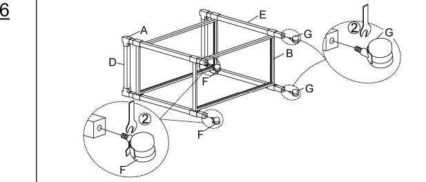
**6.1)** Attached Wheel with brakes(F) and Wheel (G) using Wrench (②) as shown above.
