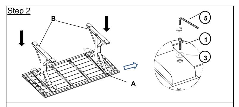
Attach Leg(B) to the Table Top(A) using Bolts(1), anh Washers (3) with Allen Key(5). **Do not fully tighten the Bolts.**
