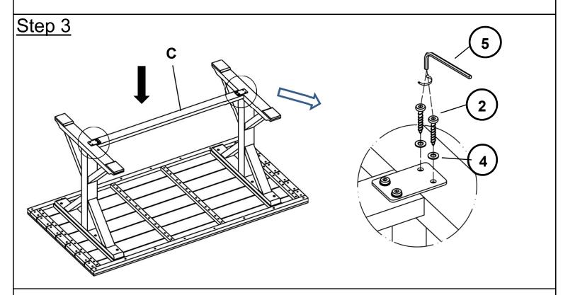
Attach the Horizontal bar (C) to the leg as shown in picture.
