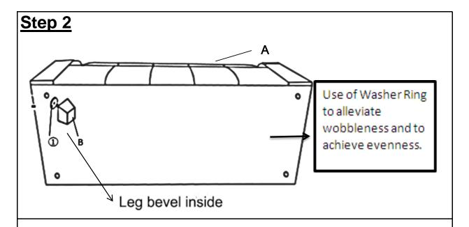
Install the first leg(B) into the bottom of the Storage Ottoman(A) by placing 1 (ONE) piece of Washer Ring on the threaded stem. The use of Washer Rings improves tightness and security of leg after assembly.
