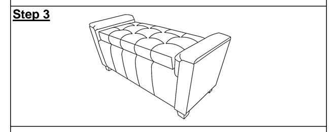
Place the Storage Ottoman right side up, test for eveness. Where you find this Storage Ottoman being uneven, identify the corresponding leg and "add or remove" a Washer Ring to achieve evenness.
