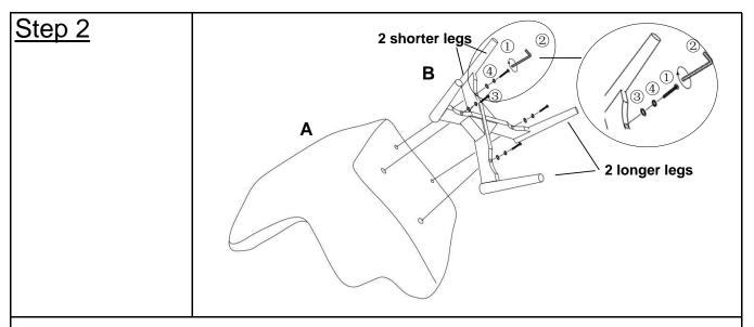
Attach Chair Base(B) onto the bottom of the Chair(A) using Bolts(1), Spring Washers(4), Washers(3) with Allen Key(2).
