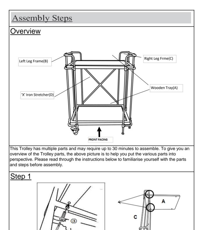
Open the carton and place all parts onto a clean, non-marring surface. Place the Right Leg Frame(C) on it's side as shown. Attach the top Wooden Tray(A) to the Right Leg Frame(C) using Bolts(③) with Allen Key(④). **Do not fully tighten the Bolts.**
