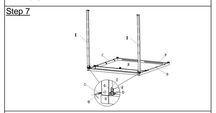
Attach Bottom Tube(I) to Main Pillar(C) and Main Pillar(D) using Bolts(1) with Allen Key(6). Attach Bottom Tube(I) to Main Pillar(C) and Main Pillar(D) using Bolts(4) and Washers(5) with Allen Key( $\Im$ ) as shown above.
