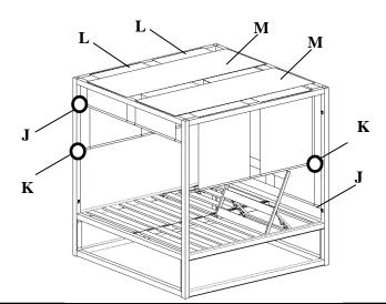
Insert the Pull Tubes(J) into the sleeves of the Canopies(M). Insert the Pull Tubes(K) into the sleeves of the Canopies(L).
