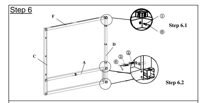
**6.1**Attach Main Pillar(D) to Supporting Fabric Tube(F) using Bolts(①) with Allen Key(⑥) as shown above
