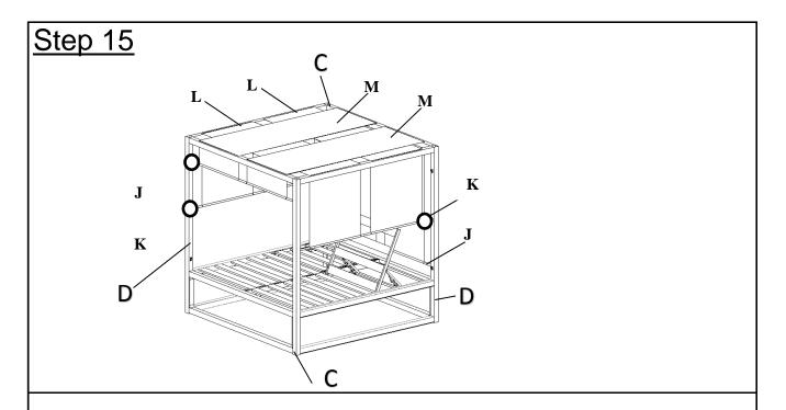
Insert Pull Tubes(J/K) into Main Pillars(C) and Main Pillars(D) holding clips as pictured.
