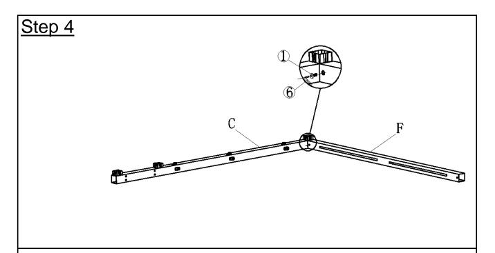
Attach Main Pillar(C) to Supporting Fabric Tube(F) using Bolts(1) with Allen Key(6) as shown above.
