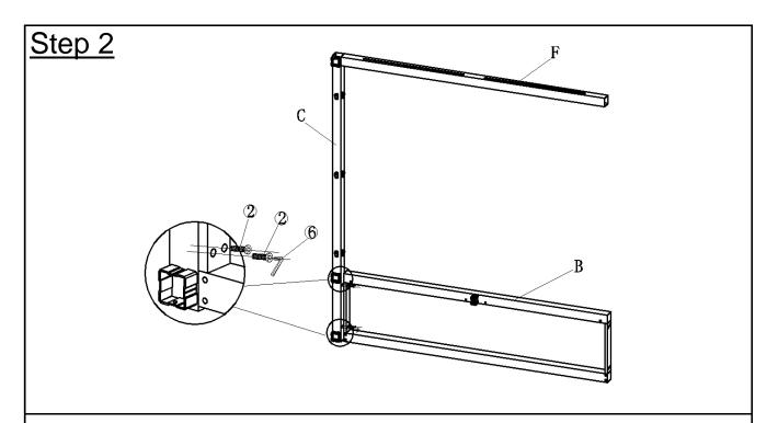
Attach Back Leg(B) to Main Pillar(C) using Bolts(②) with Allen Key(⑥) as shown above **Do not fully tighten the Bolts.**
