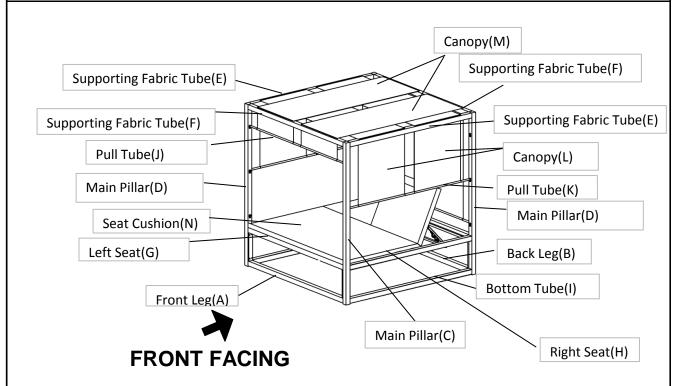
This Gazebo has multiple parts and may require up to 3-4 hours to assemble. To give you an overview of the Gazebo parts, the above picture is to help you put the various parts into perspective. Please read through the instructions below to familiarise yourself with the parts and steps before assembly.
