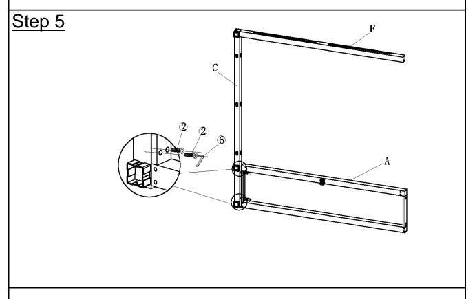
Attach Front Leg(A) to Main Pillar(C) using Bolts(②) with Allen Key(⑥) as shown above **Do not fully tighten the Bolts.**
