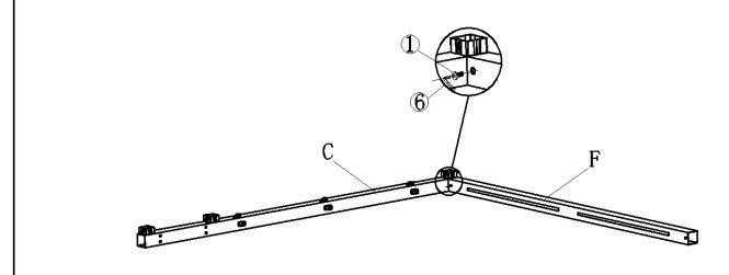
Open the carton and place all the parts onto a clean, non-marring surface. Attach Main Pillar(C) to Supporting Fabric Tube(F) using Bolts(①) with Allen Key(⑥) as shown above.
