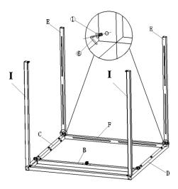
Attach Supporting Fabric Tube(E) to Main Pillar(C) and Right Main Pillar(D) using Bolts(1) with Allen Key(6) shown above.
