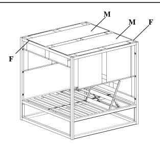
Insert the Canopies(M) through Supporting Fabric Tubes(F) as shown above
