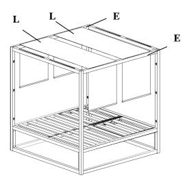
Insert the Canopies(L) through Supporting Fabric Tubes(E) as shown above
