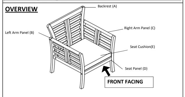
This **Armchair** has multiple parts and may require up to some 30 minutes to assemble. To give you an overview of the **Armchair** parts, the above picture is to help you put the various parts into perspective. Please read through the instructions here below to familiarise the parts and steps before assembly.
