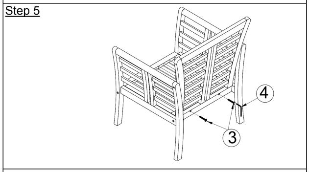
Use Short Screw (3) and Allen Wrench (4) to attach Backrest Panel (A) and Seat Panel (D).
