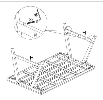
With the help of your adult partner attach the Support Leg (H) to the Right Leg (F) and Left Leg (G) using Screws (④) with Allen Wrench (⑤)as shown in the picture above.
