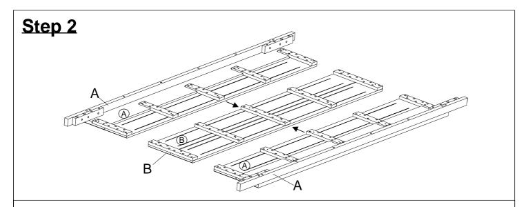
Place the Side Table Top Panel (A) and Middle Table Top Panel (B) on the surface as shown above. Attention: Labels (A), (B) sticked on these parts are supposed to be on the same side once assembly as pictures shown above.
