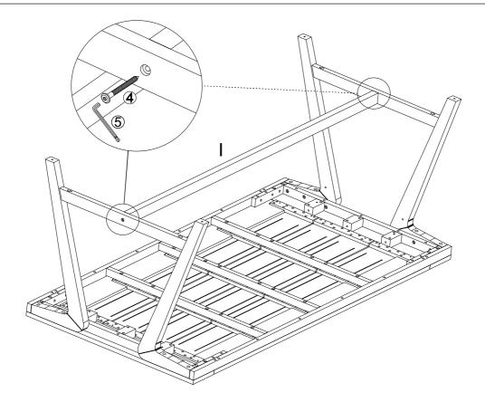
With the help of your adult partner, attach the Support Bar (I) to the Support Leg (H) using Screws (4) with Allen Wrench(5)as shown in the picture above.
