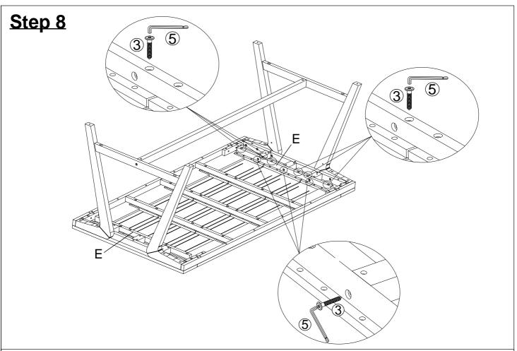
Attach the Side Support Top (E) to the Side Table Top Panel (A), Middle Table Top Panel (B) and Table wings Panel (C1, C2) using Screws (③) with Allen Wrench(⑤) as shown in the picture above. Repeat the same process with the Side Support Top (E) second.
