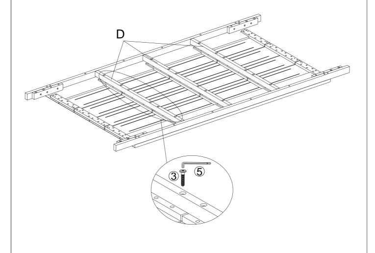
Attach the Middle Support Top (D) to the Side Table Top Panel (A) and Middle Table Top Panel (B) using Screws (③) with Allen Wrench (⑤) as shown in the picture above. **DO NOT fully tighten the Screws.**
