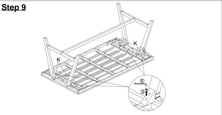
Attach the Corner (K) to the Right Leg (L), Left Leg (G) and Table wings Panel (C) using Screws ( $\Im$ ) with Allen Wrench ( $\Im$ ) as shown in the picture above.
