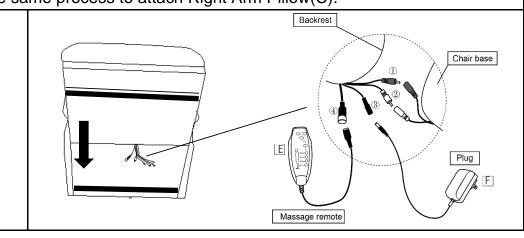
No.1 and No.2 wire connect with the Chair Backrest(A) and Chair Base(D). (Two same color wires connect)
