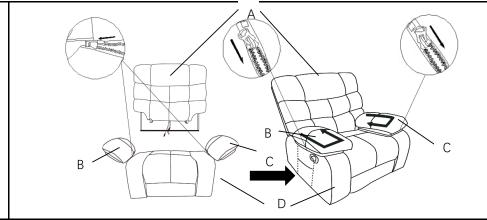
Attach the Left Arm Pillow(B) using the prefabricated Zipper. Repeat the same process to attach Right Arm Pillow(C).
