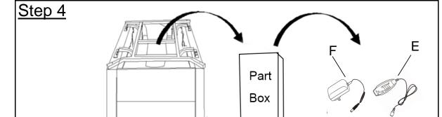
Take out the accessories box from the bottom of the mechanism. Then remove the Massage Remote(E) and Plug(F) from the accessories package.
