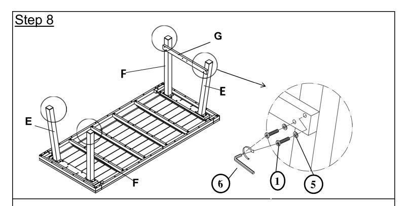
Attach the First Leg Support Bar(G) to First Leg(E) and Second Leg(F) using Bolts( $\bigcirc$ 1), and Washers( $\bigcirc$ 5) with Allen Wrench( $\bigcirc$ 6) as shown above.
