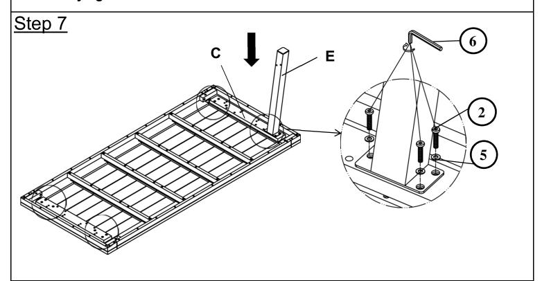
Attach First Leg(E) to End Table Top(C) using Bolts((2)), and Washers((5)) with Allen Wrench((6)) as shown in the picture above.
