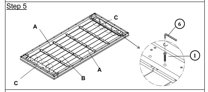
Attach End Table Tops(C) to Side Table Tops(A) and Center Table Top(B) using Bolts(1))with Allen Wrench(6) as pictured above.
