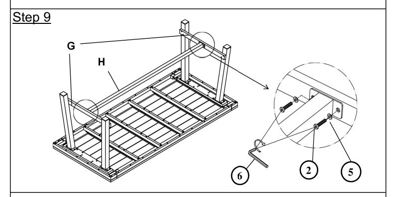
Attach Second Leg Support Bar(H) to First Leg Support Bar(G) using Bolts(2), and Washers(5) with Allen Wrench(6) as pictured above.
