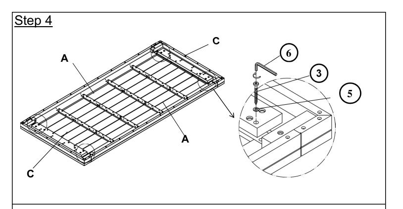
Attach End Table Top(C) to Side Table Tops(A) using Screws(3), and Washers(5) with Allen Wrench(6) as pictured above.
