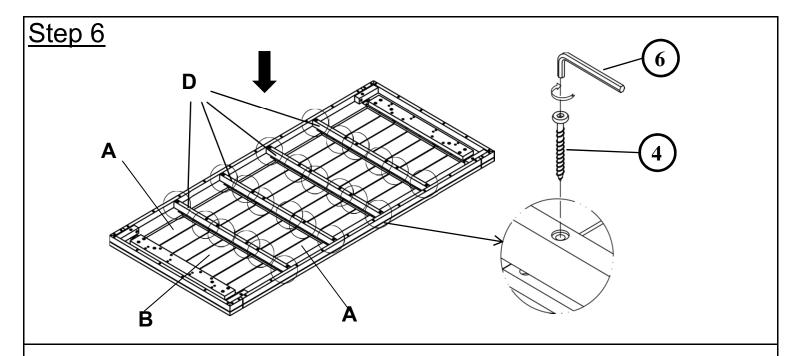
Attach Table Support Bars(D) to Side Table Tops(A) and Center Table Top(B) using Screws(4) with Allen Wrench(6) as pictured above.
