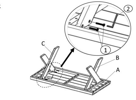
Attach Left Leg(C) to Table Top(A) by using 2 Bolts(1) with Allen Wrench(2) as indicated. **Do not fully tighten the Bolts.**
