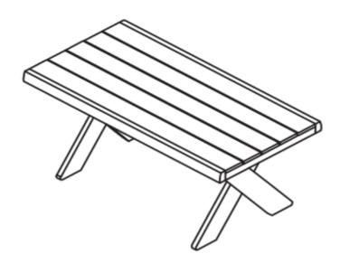
Place the Table onto a level surface, then EXERT pressure, floorwards, onto the Table. This pressure will help the Legs and Table Top reach full alignment at all joints.
