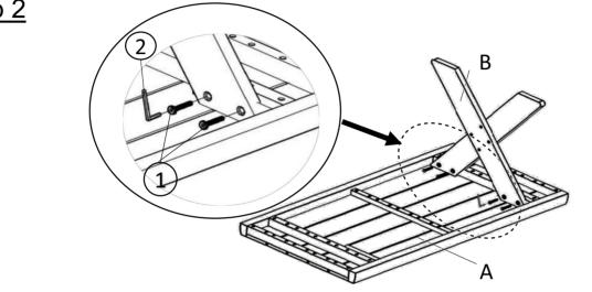
Attach Right Leg(B) to Table Top(A) by using 2 Bolts(①) with Allen Wrench(②) as shown above.
