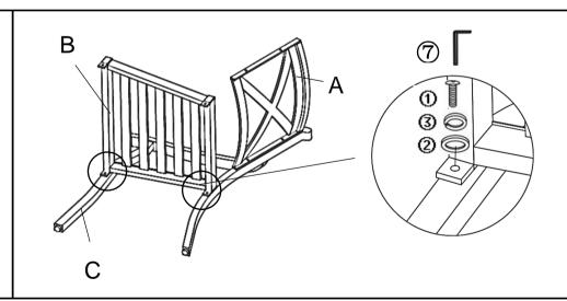
Then attach Chair Seat Panel(B) to Left Arm Leg with Pre-attached Levellers(C) using bolts(1), spring washers(3) and washers(2) with allen key(7).
