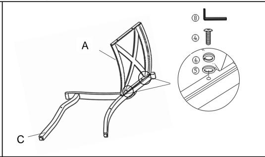
Turn the Left Arm Leg with Pre-attached Levellers(C) upside down on to a soft surface.
