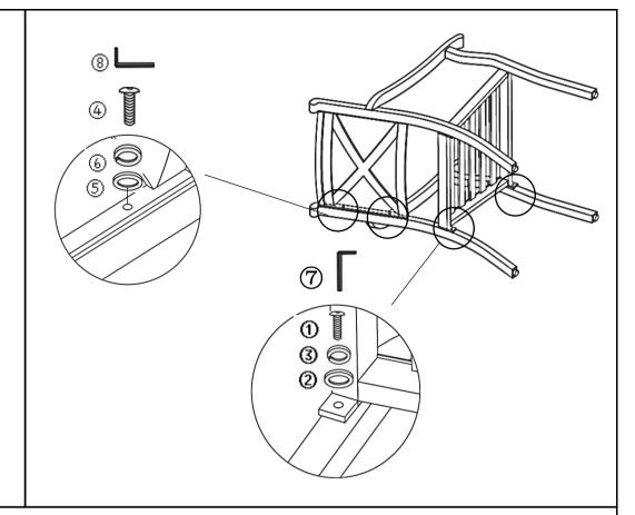
Repeat the same assembly process for the Right Arm Leg with Preattached Levellers(D).
