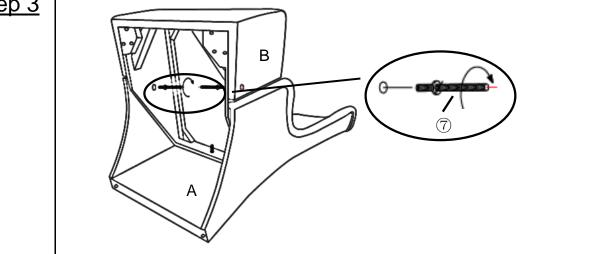
Connect Chair Back(A) with Seat(B) using Screw Arbor(①) and tightening tighten by turning the Screw Arbor(①) clockwise, as shown.
