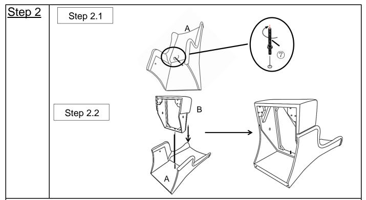
Step 2.1 Screw the Screw Arbor(⑦) into Chair Back(A) by turning clockwise as shown.
