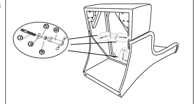
Align the mounting positions on the right ,middle and left of Chair Back(A) and Seat(B); using the Spring Washers(5), Washers(3), Nut(9) mounted on Screw Arbor(7) with Spanner(8).
