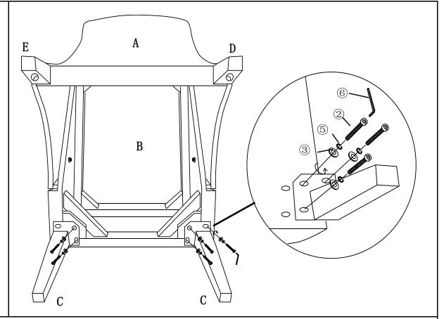
Align the mounting positions of Front Legs(C) to Seat(B), then attach using Bolts(2), Spring Washers(5) and Washers(3) with Allen Key(6).
