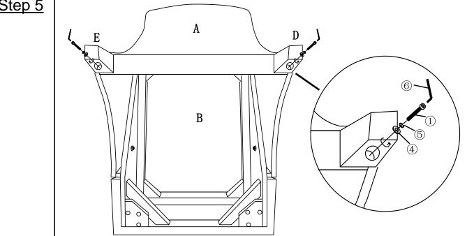
Attach Back Leg(D) to the bottom of the Chair Back(A) using Bolt(1), Spring Washer(5) and Washer(4) with Allen Key(6).
