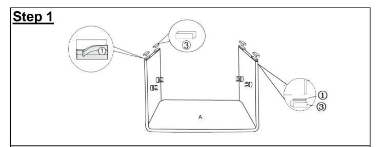
Put Coffee Table Main Frame(A) face down carefully onto a soft, non-marring surface.
