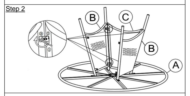
Attach Leg Support Panel(C) between Leg Panels(B) using Bolts( $\Im$ ) and Washers( $\Im$ ) with Allen Key( $\Im$ ) as shown in the picture above.
