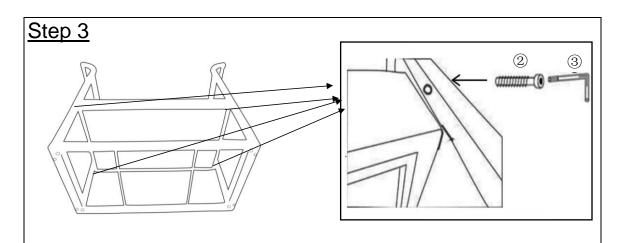
Attach middle Tray(D) between Side Panels with Handrail(C) using Bolt(②) with Allen Wrench(③).
