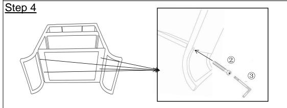
Attach Top Shelf(A) to between Side Panels with Handrail(C) using Bolt(2) with Allen Wrench(3).
