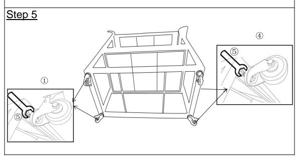
Turn-in Wheels(①&④) using Spanner(⑤), into the four Mounting Positions. Note: There are two wheels have braking functions, you must keep this two wheels installed in the same end. To activate the Brake press the Lever down. To release the Brake lift the Lever up.
