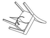
Finally, seal the Seat Base Cover back on to the underside of the chair seat . Turn it the right side up.The chair is ready for use.
