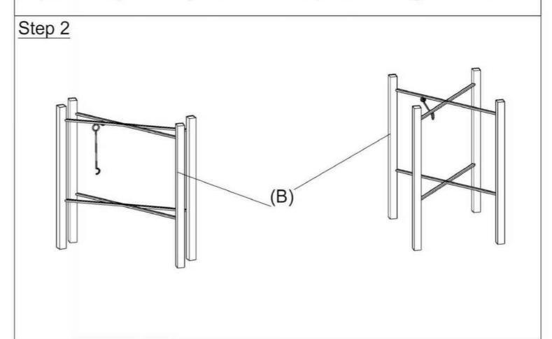
Hold up the collapsable Iron Base (B) as shown above and fix it with attached latch
