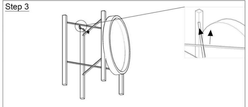
As shown above, the arrow mark underneath the Tray should be placed upright with the arrow mark on the iron base.
