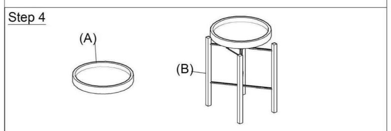
Place the wooden End Top (A) on the Iron Base (B) as shown above.
