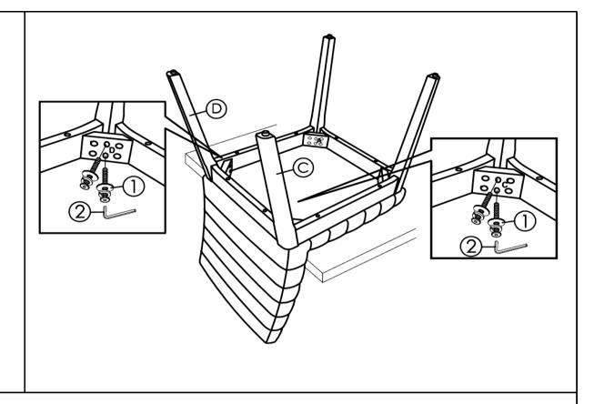
Repeat Step 1, to place the Back Leg (C) and Back Leg (D) in the other corner blocks as shown.
