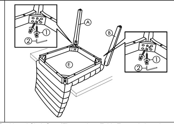
Place the Cushioned Chair Seat (E) on a clean Table Top and place the Front Leg (A) Front Leg (B) on the corner block as shown.
