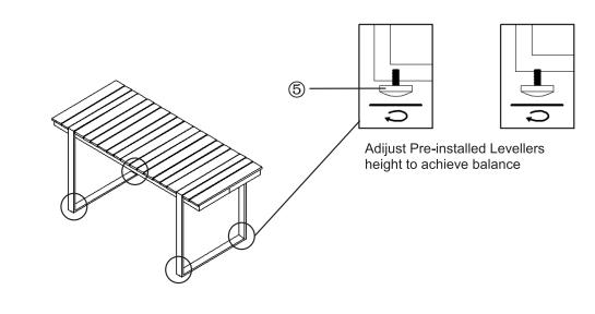
Insert the adjusting foot pad (⑤) into the Leg tube(A), as shown in the figure above. Table is ready for use.
