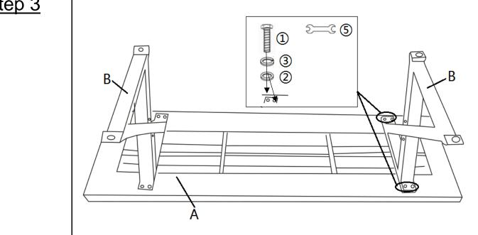
Attach Chair Leg with Pre-attached Levellers(B) to Seat Plate(A) using Washers(2), Spring Washers(3), and Hex Bolts(1) with Spanner(5). Do not fully tighten the Bolts.
