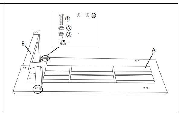
Attach Chair Leg with Pre-attached Levellers(B) to Seat Plate(A) using Washers(2), Spring Washers(3), and Hex Bolts(1) with Spanner(5). Do not fully tighten the Bolts.
