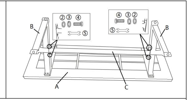
Attach Supporting Rod(C) between Chair Legs with pre-attached Levellers(B) using Washers(2), Spring Washers(3) and Hex Bolts(4) with Spanner(5).
