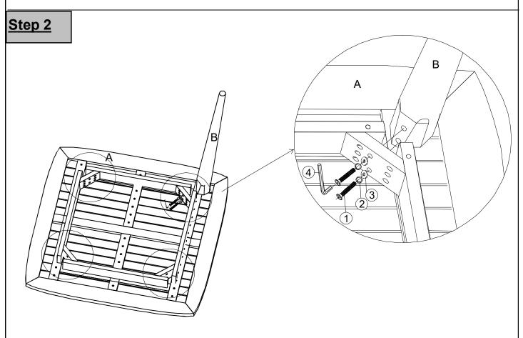
Attach Leg (B) to the Table Top (A) by using 2 Bolts (1), 2 Spring Washers (2) and 2 Washers (3) with Allen Wrench (4).
