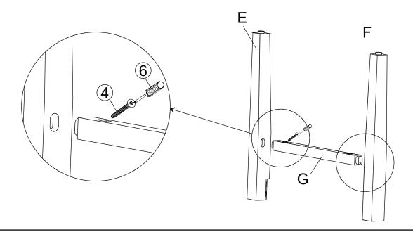
Attach Front Support Bar(G) into the upper housing of the Top Right Front Leg (E) and Top Left Front Leg (F).
