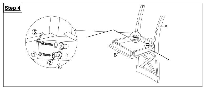
Place the Chair Seat (B) onto the side of a table or a box as shown in above picture. You will have the Chair bottom and legs facing skywards.
