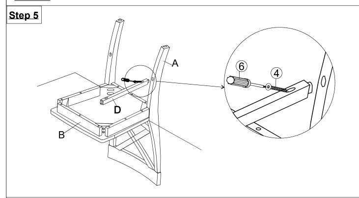
Next, place Left Side Rail (D) into the oval housing of Hind Leg of the Chair Back (A) as shown in the picture.
