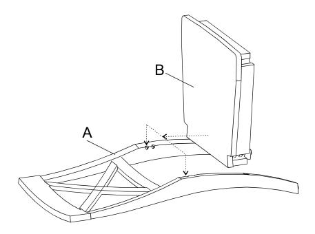
Place the Chair Back (A) onto a flat clean soft surface, as pictured above Push the Chair Seat (B) in to the mounting position of the Chair Back (A) following the arrows shown in the picture.
