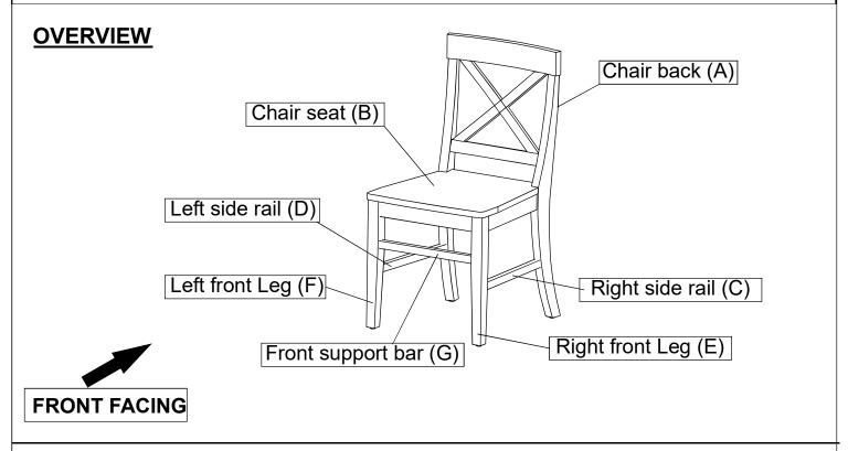
This Chair has multiple parts and may require up to some 30 minutes to assemble. To give you an overview of the Chair, the above picture is to assemble is to help you put the various parts into perspective. Please read through the instructions here below to familiarise the parts and steps before assembly.
