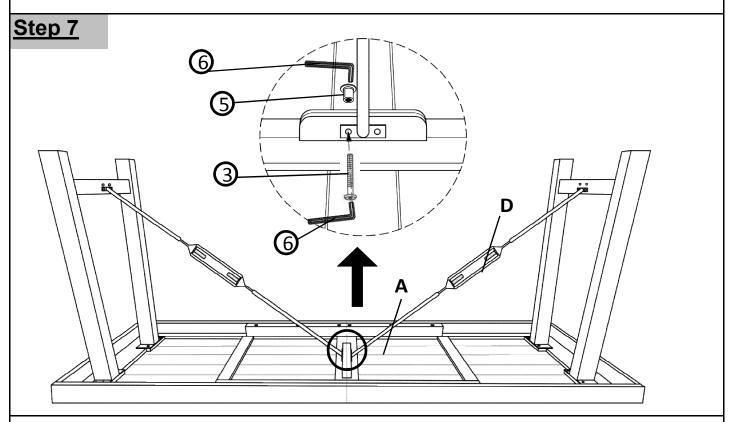
Affix Side Turnbuckle Set(D) to Table Top(A) using Long Bolt(3) and Sleeve Nut(5) with Allen Wrench(6).
