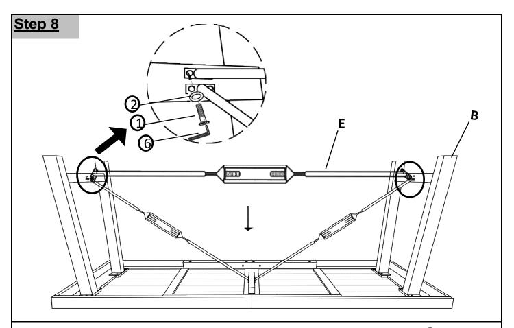
Attach the Bottom Turnbuckle Set(E) to Iron Legs(B) using Short Bolt(1) and Washer(2) with Allen Wrench(6).
