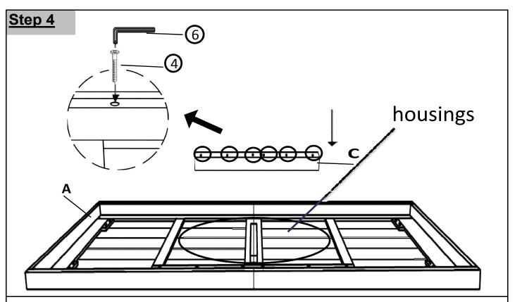
Align Support Bar(C) to the housings on Table Top(A) and secure using Screws(4) with Allen Wrench(6).
