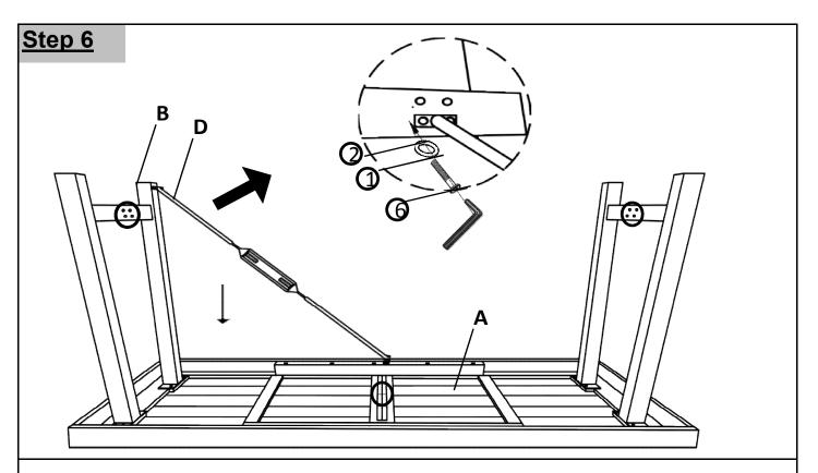
Place Side Turnbuckle Set(D) between housing of Table Top(A) and Iron Leg(B). Attach Side Turnbuckle Set(D) to Iron Leg(B) using Short Bolt(1) and Washer(2) with Allen Wrench(6)
