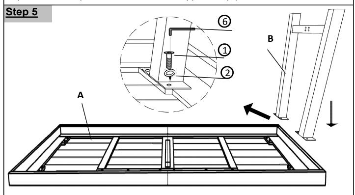
Attach Iron Leg(B) to Table Top(A) using Short Bolt((1)) and Washer((2)) with Allen Wrench((6)).
