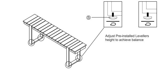
Insert the adjusting foot pad (5) into the Leg tube(A) , as shown in the figure above. Bench is ready for use.
