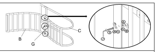
Join the three mounting positions of the Back Frame(B) and the Seat Frame(C) together using the Connecting Plate(G), Bolts(3), Spring Washers(4), Washers(5) and Nuts(6), utilizing the Allen Wrench(7) to tighten the bolts on the top side, then use the Wrench(8) to tighten on the back as pictured.
