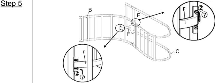
Attach the Back Supporter(F) to the Back Frame(B) and the Connecting Slat(E) using Bolts(2) and the Allen Wrench(7) as pictured. Pay attention to attach the end marked "B end" to the Back Frame(B) and attach the end marked "E end" to the Connecting Slat(E). Fully tighten the Bolts in a sequential manner.
