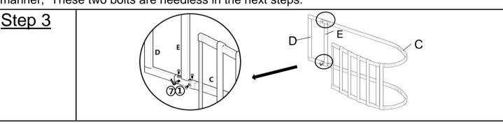
Place the Seat Frame(C) and the Extension Panel(D) on its side as pictured. Attach the Extension Panel(D) to the Seat Frame(C), then join them together using the Connecting Slat(E), 4 Bolts(①) on each side, and the Allen Wrench(⑦) as shown above. Fully tighten the Bolts in a sequential manner.
