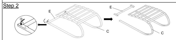
Place the assembled Connecting Slat(E) and Seat Frame(C) as pictured. Disassemble the Connecting Slat(E) from Seat Frame(C) by using Allen  $Wrench(\mathfrak{T})$  in a anticlockwise manner, These two bolts are needless in the next steps.
