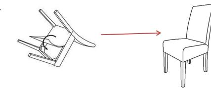
Finally, seal the Seat Base Cover back on to the underside of the chair seat . Turn it the right side up.
