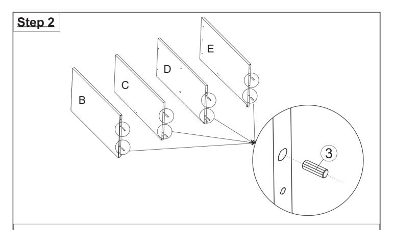
By hand, attach Wooden Dowel (③) to Left Panel (B), Left Floor Panel (C), Right Floor Panel (D), Right Panel (E) as shown above
