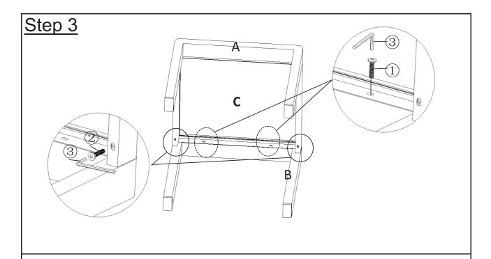
Attach Table Top Frame(C) to Right Leg(B) using Bolts(1) and Bolts(2)with Allen Wrench(3) as shown in the picture.
