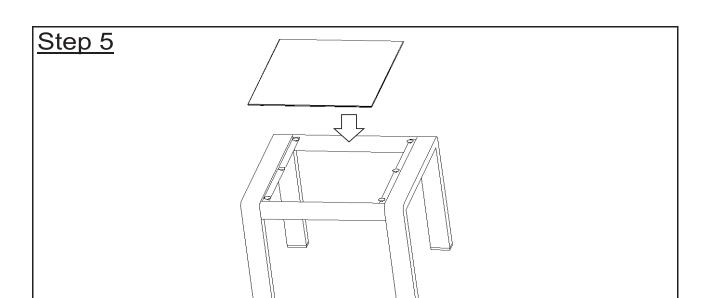
Place the Glass Top(D) on the assembled Table Frame.
