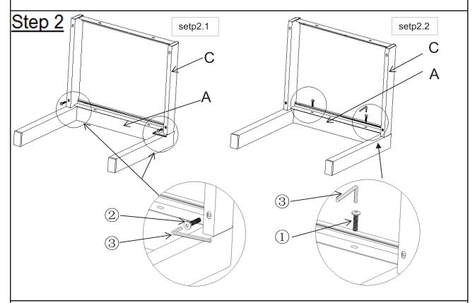
Step2.1: Attach the Table Top Frame(C) to the Left Leg(A) using Bolts(②) with Allen Wrench(③) as shown in the picture.
