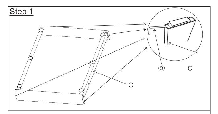
Take out the guards in the four ends of Table Top Frame(C) using Allen Wrench(③).
