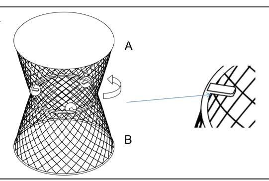
Rotate the Top(A) along the Base(B) until the Tapers lock into place.
