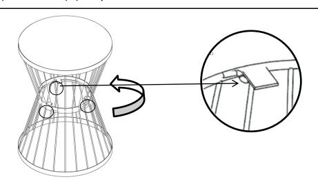
Rotate the Top(A) along the Base(B) until the Tapers lock into place.
