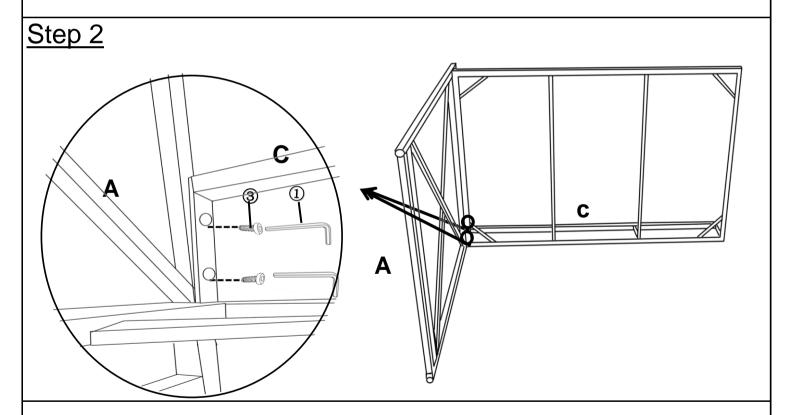
Attach Top Shelf Frame(C) to Left Frame(A) using Bolts( $\Im$ ) with Allen Key( $\Im$ ). **Do not fully tighten the Bolts.**
