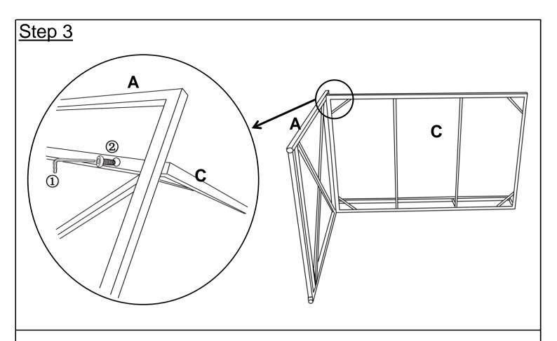
Attach Top Frame(C) to Left Frame(A) using Bolts(2) with Allen Key(1). **Do not fully tighten the Bolts.**
