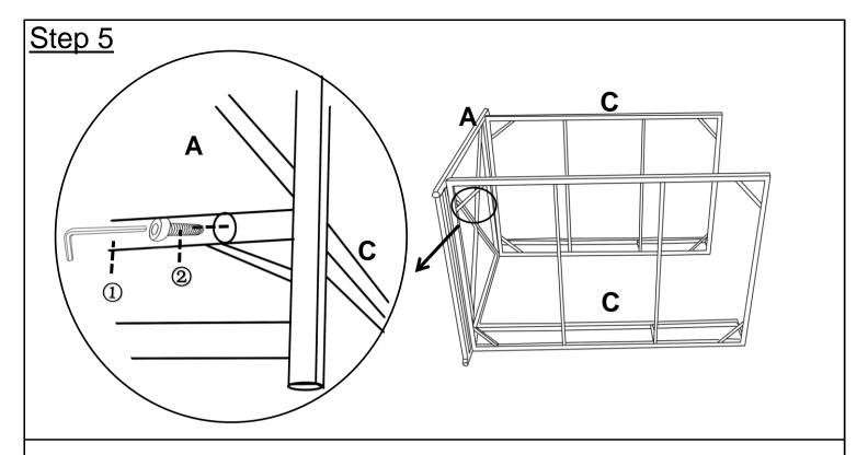
Attach Top Frame(C) to Left Frame(A) using Bolts(2) with Allen Key(1). Do not fully tighten the Bolts.
