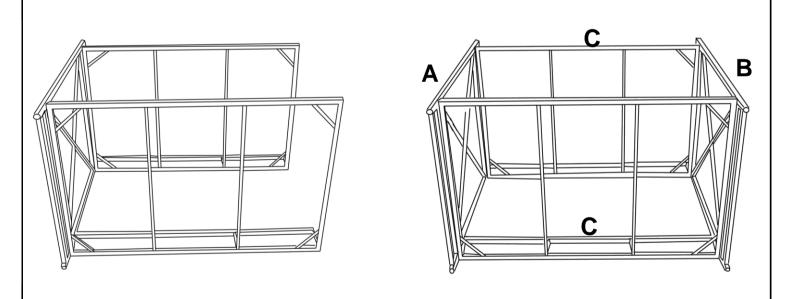
Repeat Steps 2 - 5 to assemble Right Frame(B). Do not fully tighten the Bolts.
