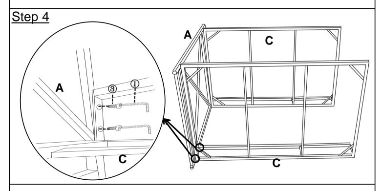
Attach Bottom Frame(C) to Left Frame(A) using Bolts( $\Im$ ) with Allen Key( $\Im$ ). **Do not fully tighten the Bolts.**
