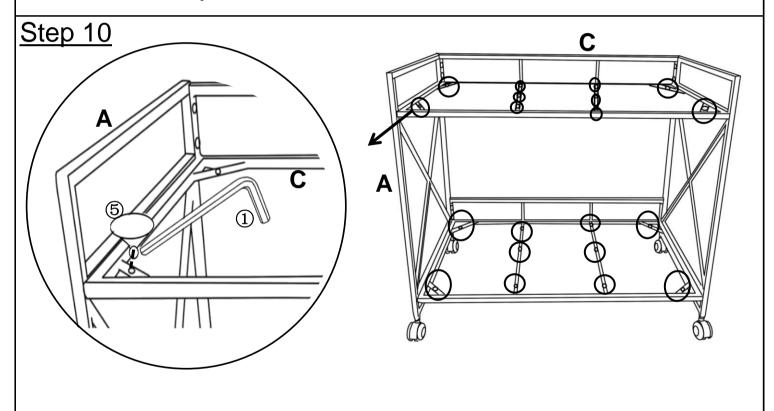
Attach Glass Suction Cup(5) to Top Shelf Frame(C) and Bottom Frames(C), as shown. You can press the Glass Suction Cup(5) with Allen Key(1) if donot assemble easily .
