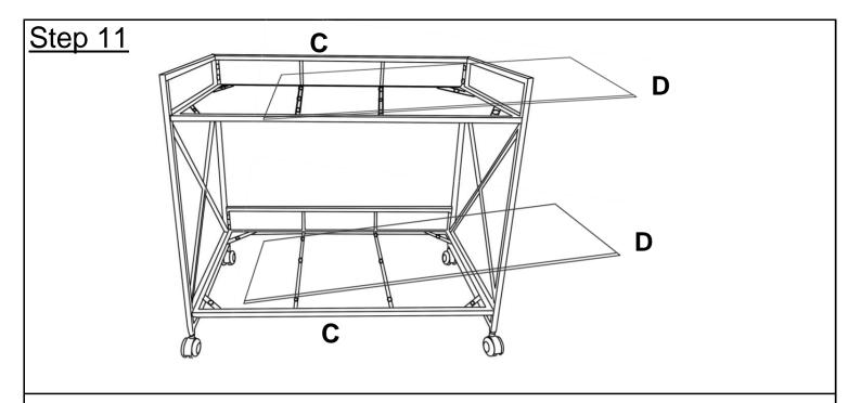
Insert Top Glass(D) into Top Shelf Frame(C) and Bottom Glass(D) into and Bottom Frame(C) Carefully.
