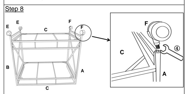
Attach Wheels with Brakes(F) to Left Frame(A) using Spanner(4). Attach Wheels(E) to Right Frame(B) using Spanner(4).
