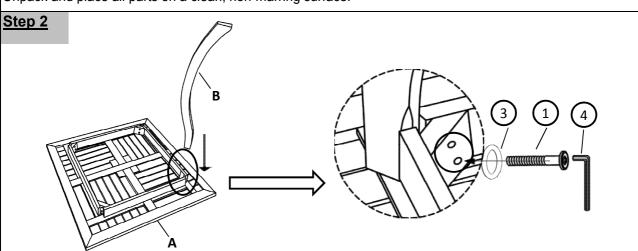
Attach Leg(B) to the Table Top(A) using Bolt (1) and Washer(3) with Allen Wrench(4). Only loosely tighten the Bolts.
