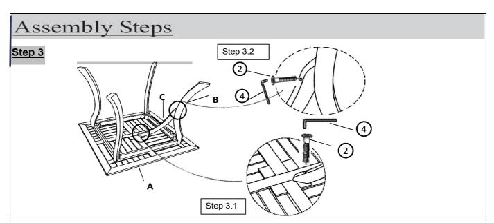
Place Leg Support(C) between Table Top(A) and Leg(B), as shown above
