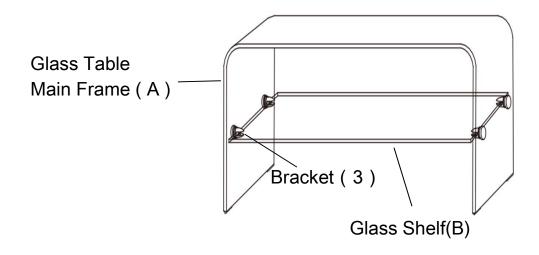
This Glass Table has multiple parts and may require up to some 5-10 minutes to assemble. To give you an overview of the Table parts, the above picture is to help you put the various parts into perspective. Please read through the instructions herebelow to familiarise the parts and steps before assembly.
