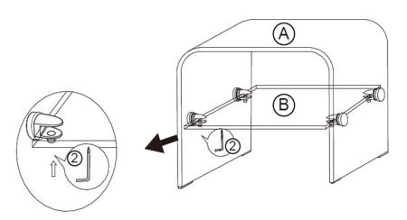
Carefully insert Glass Shelf(B) into the Brackets on the Glass Table Main Frame (A). Tighten the Plastic Bolts at the bottom of the Brackets until the Glass Shelf is secured in place.
