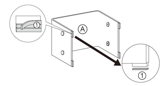
Put Glass Table Main Frame (A) carefully on its side onto a soft, non-marring surface. Peel a Pad(1) off the backing and apply it squarely to an Aluminum Leg as shown in the picture. Repeat this step with the remaining three feet.
