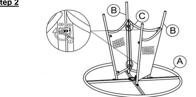
Attach Leg Support Panel(C) between Leg Panels(B) using Bolt(3) and Washer(2) with Allen Key(1) as shown in the picture above.
