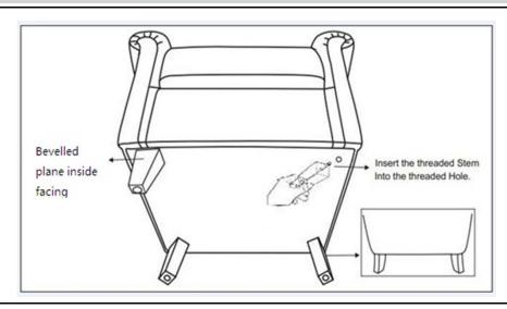
Install the first leg into the bottom of the chair by placing 1 plastic washer ring (improves tightness and security of leg) onto the threaded stem.
