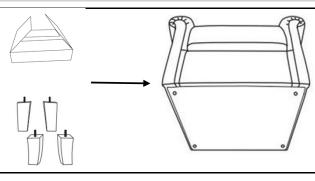
Position the Chair on its back, as shown on a surface that won't scratch the upholstery. Open the inner box and take out the 4 Wooden Legs provided
