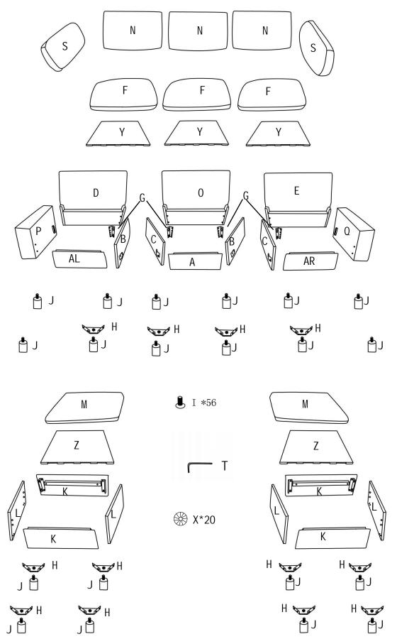
Connect Left armrest(Part P) and Left backrest(Part D) with the insert. Hang Hinge (Hardware G) on the screws of Right baffle(Part B), connect Left backrest(Part D) and Right baffle(Part B) with Screws(Hardware I), and tighten the screws with Simple screwdriver(Hardware T). Hang Left front baffle(Part AL) on the screws of Left armrest (Part P) and Right baffle(Part B) respectively, tighten the screws, and the left seat frame is connected.
