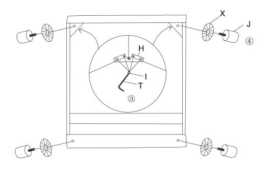
Connect Right armrest(Part Q) and Right backrest(Part E) with the insert. Hang Hinge (Hardware G) on the screws of Left baffle(Part C), connect Right backrest(Part E) and Left baffle(Part C) with Screws(Hardware I), and tighten the screws with Simple screwdriver(Hardware T). Hang Right front baffle(Part AR) on the screws of Right armrest (Part Q) and Left baffle(Part C) respectively, tighten the screws, and the Right seat frame is connected.
