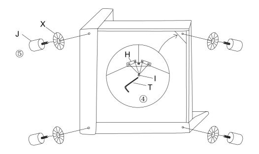
Hang Hinges(Hardware G) on the screws of Left baffle(Part C) and Right baffle(Part B), connect Right baffle(Part B) and Middle backrest(Part O), Left baffle(Part C) and Middle backrest(Part O) with Screws(Hardware I), and tighten the screws with Simples crewdriver (Hardware T). Hang Middle front baffle(Part A) on the screws of Left baffle(Part C) and Right baffle(Part B) respectively, tighten the screws, and the middle seat frame is connected.
