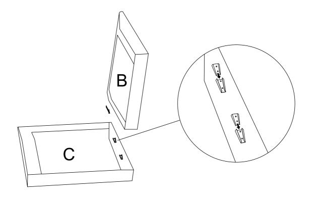
Use all hardwares listed in the upper right table to connect the Seat frame(part D), the Arm (part B) and the Backrest (part C). Put the Spring wahsers (part 3) on top of the flat washer (part 2). Don't screw any bolt all in until the others are all put into the holes. To ensure the good looking of the chaise, remember to keep the buttom of the frame align. Tighten all the bolts.
