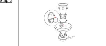
Through pump wire into PVC pipe in the fountain part A, then pull it out of the bottom of fountain part A.
