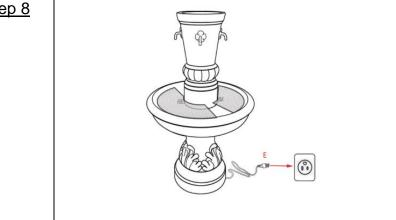
Plug the pump (E) in the socket showed as above. The water will start to flow in minutes.
