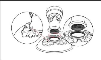
Place the fountaina body B upside down on a level surface away from areas where it is likely to get colgged with leaves and make sure that the cable will reach the socket, then turn fountain body A into fountain body B (anticlockwise). The sign arrow must align after assembling.
