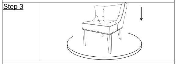
Place the chair on a LEVEL SURFACE to see if it wobbles. If it wobbles, press firmly down on both armrests at the same time. This will help to ensure all Bolts and gaps reach full alignment status. If no wobbles found, proceed to tighten all the Bolts. DO NOT fully tighten a BOLT in one go and then move on to the next. Rather, in a sequential manner, gradually tighten each Bolt until all Bolts are evenly secured.
