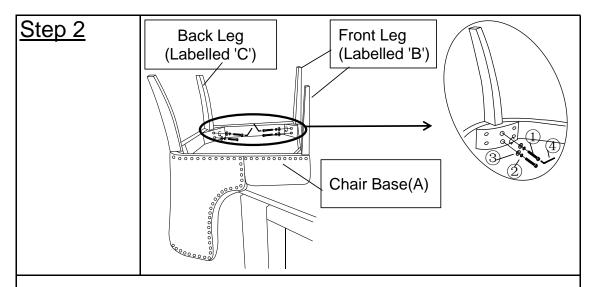
Insert the Front Leg(B) and Back Leg(C) into the mounting position of Chair base(A).
