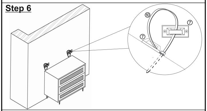
Move Cabinet to the wall. Pull the Restraint Straps (®) through the Brackets(¬) on the wall and Cabinet one by one, and pull the Restraint Strap (®) tight.
