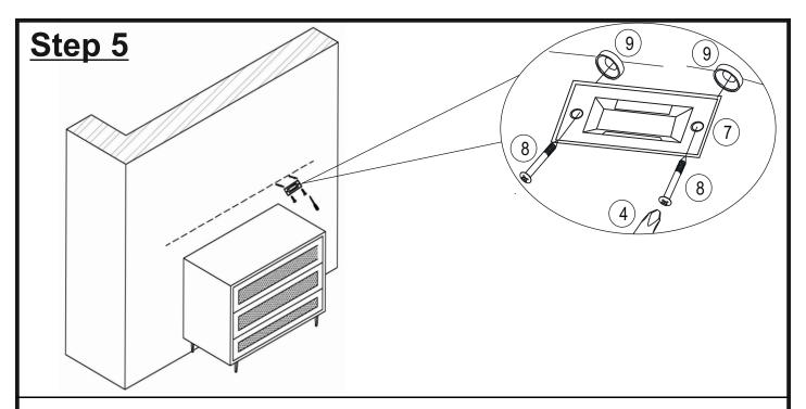
Attach Brackets(7) to Wall Plugs (9) using Wall Plug Screws (8) with Screwdriver (4).
