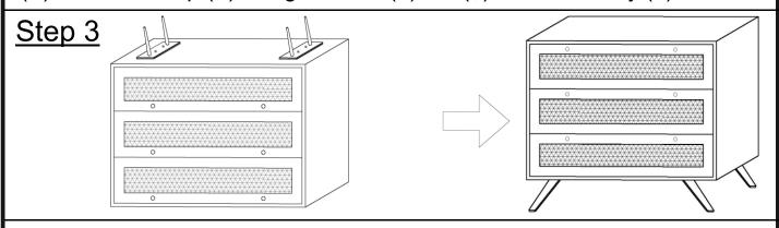
Repeat "Step2" to assemble the other Leg (B) to Cabinet top (A). Upon assembly of all the Legs (B), flip the Cabinet ,as shown in "Step3".
