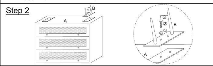
With assistance from your adult partner, place the Cabinet Top (A) face down as picture, on clean, surface. As shown in "Step2" picture attach Leg (B) to Cabinet top (A) using Washer (1), Bolt(2) with Allen Key (3).
