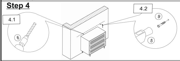
4.1) Drill two holes on wall at same height as Bracket (7) on Cabinet (A) with Power Drill (6).
